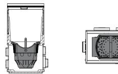
Note: Trash bucket position within SK2-621D catch basin body and base
